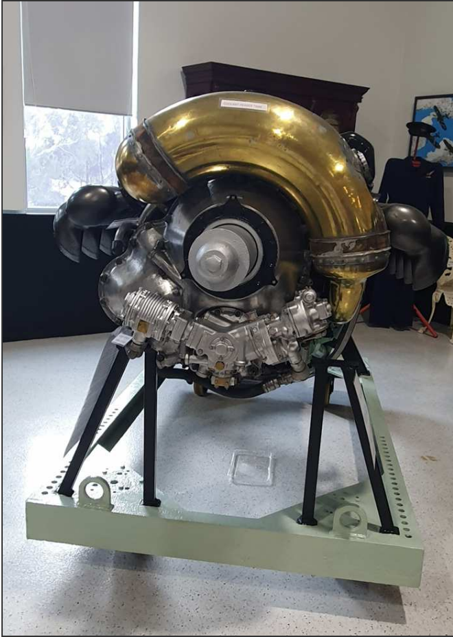
1945 Rolls-Royce Merlin V12 27 Litre Aero Engine
